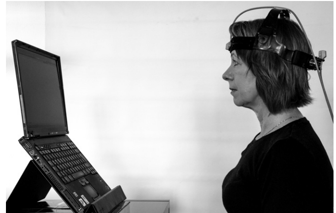
Fig. 1. Experimental set-up. The placement of the 2 sensors was on the forehead and the back of the head. The participants were seated in front of a computer screen and were asked to find their natural head posture facing forward. The distance from the participants' earlobe to the computer monitor was 100 cm.
