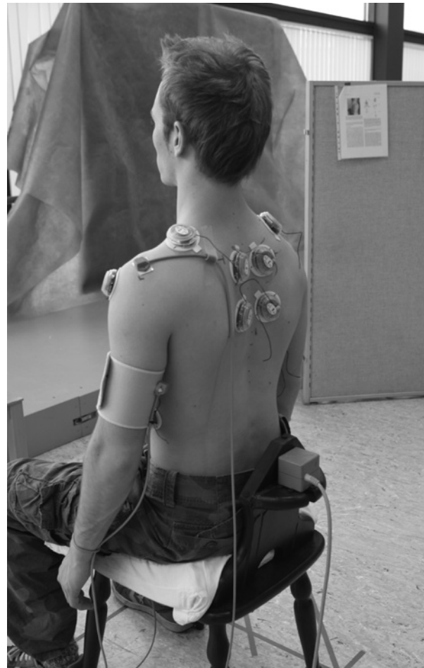
Figure 4 — Experimental setup. A sensor was attached to the skin of the sternum, to the flat part of the acromion and on the posterior aspect of the humerus. The EMG surface electrodes on the subject were not used in this study.
