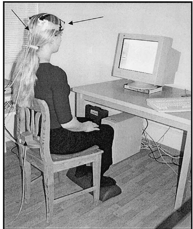
Fig 2. Experimental set-up. The subjects were seated in front of a computer and were asked to find their natural head posture. The distance from the chair back to the computer monitor was 100cm. The arrows point to the sensors attached to the head and the electromagnetic transmitter.
